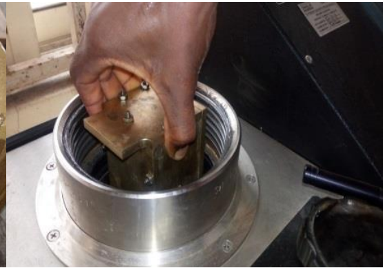
Figure 10. The brass mold in the pressure vessel
