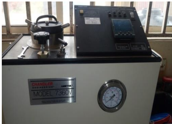
Figure 11. The pressure vessel covered by the plug.
