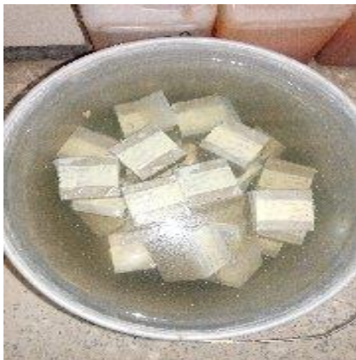
Figure 13. Further curing of produced cured cement cubes in water for 48 hours
